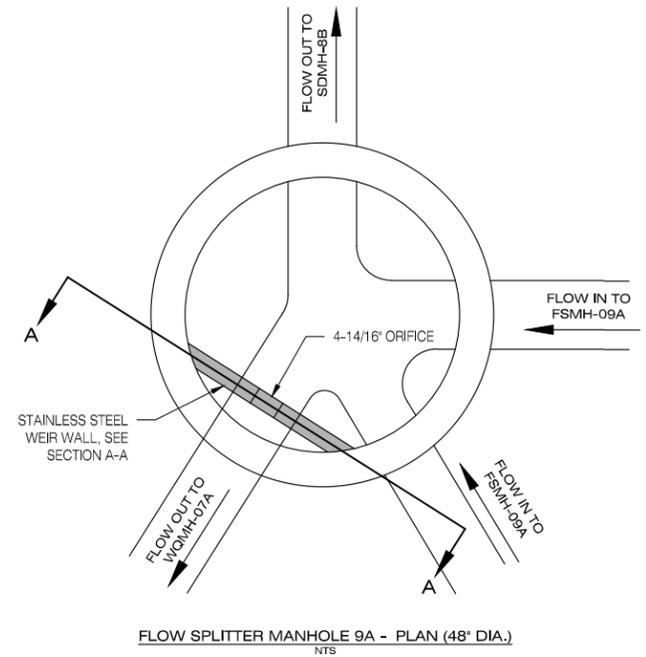
FLOW SPLITTER MANHOLE 9A - PLAN (48" DIA.)
