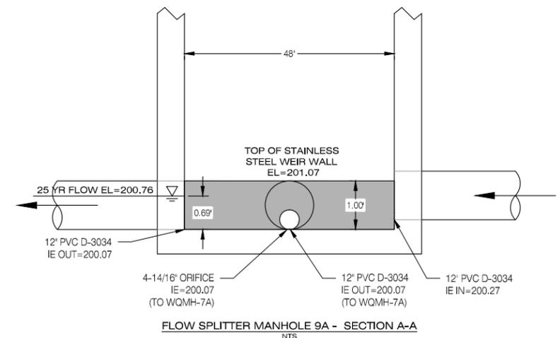
FLOW SPLITTER MANHOLE 9A - SECTION A-A
