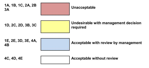
Unacceptable: The hazard must be mitigated in the most expedient manner possible before normal service may resume. Interim corrective action may be required to mitigate the hazard to an acceptable level while the permanent resolution is in development.
