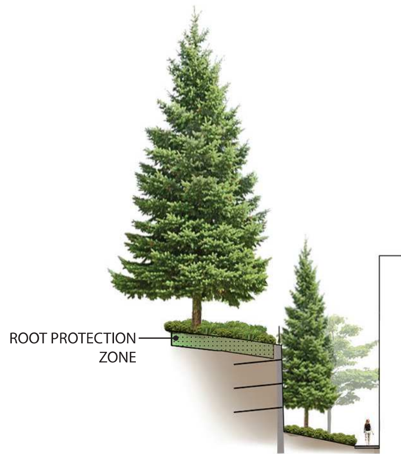
SECTION C - Option 1 PROPOSED WAIVER USING SOIL NAIL WALL
