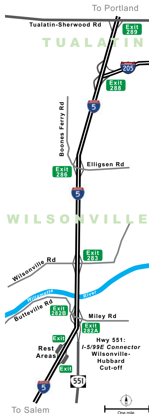
Map illustrating I-5 exits in the Wilsonville area. Each interchange on/off ramp introduces automobile weaving lane-changes that are a major contributor to traffic congestion and highway incidents.
