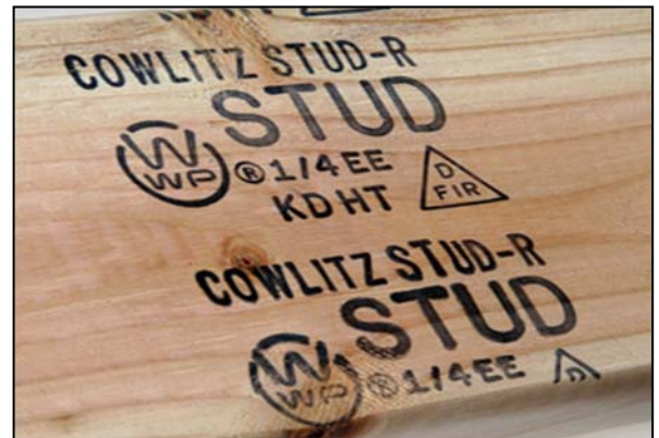
WWP markings stamped on rough sawn lumber
